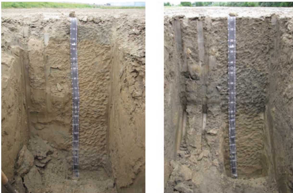
Figure 2: Two soil profile pits were dug; Profile 1 on the area where the excavated fertile topsoil was deposited directly on the agricultural land (left); Profile 2 on the area where the fertile topsoil was removed before the gravel was deposited and later restored (right)
