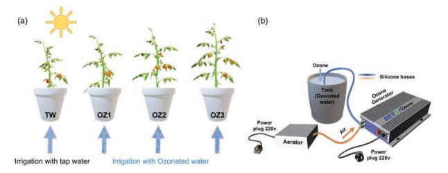
Figure 1: Experimental setup illustrating the trials
