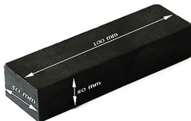
Figure 1: The geometric characteristics of the magnets used in the experiments (100×30×20 mm).
